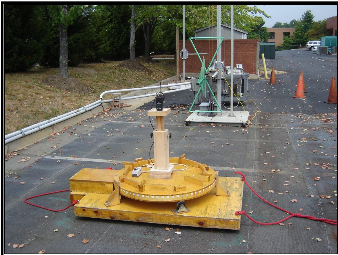
Photograph 4: Radiated TX Spurious Emissions – Front View
