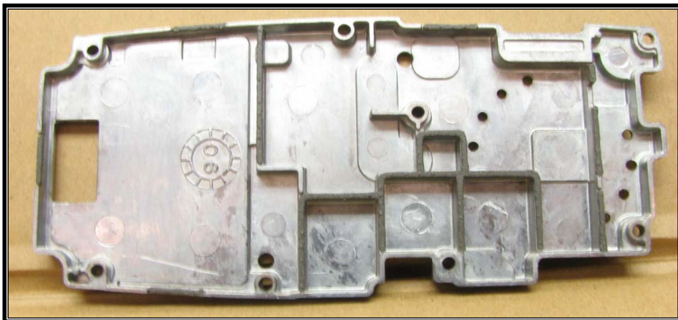
Photograph 14: RF Shield Bottom View
