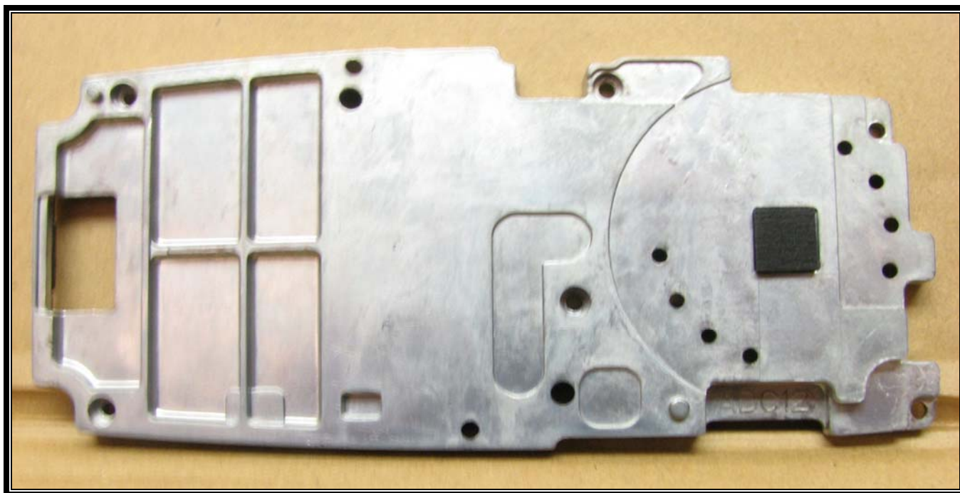
Photograph 13: RF Shield Top View
