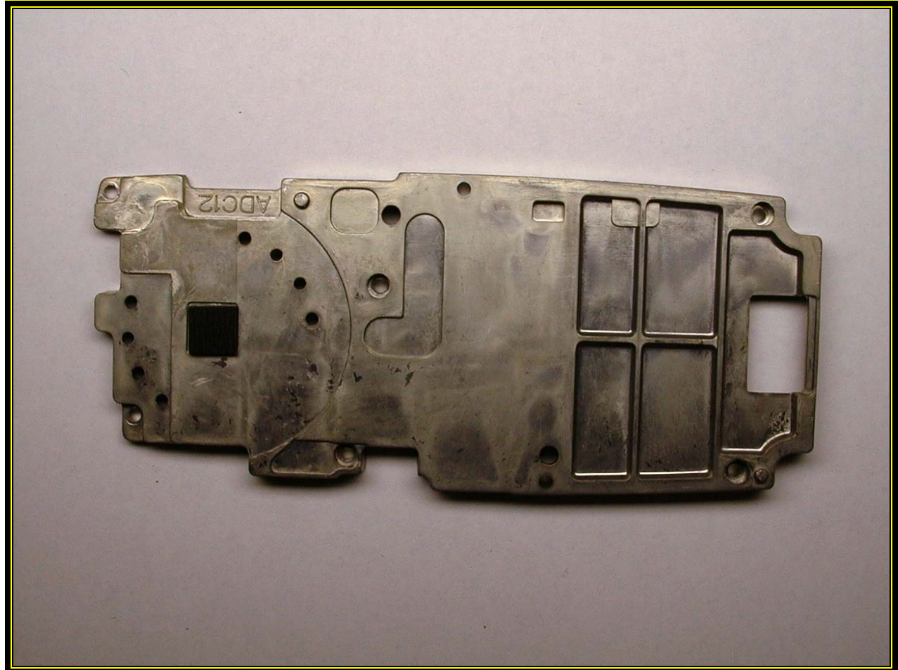
Photograph 17: RF Shield Front
