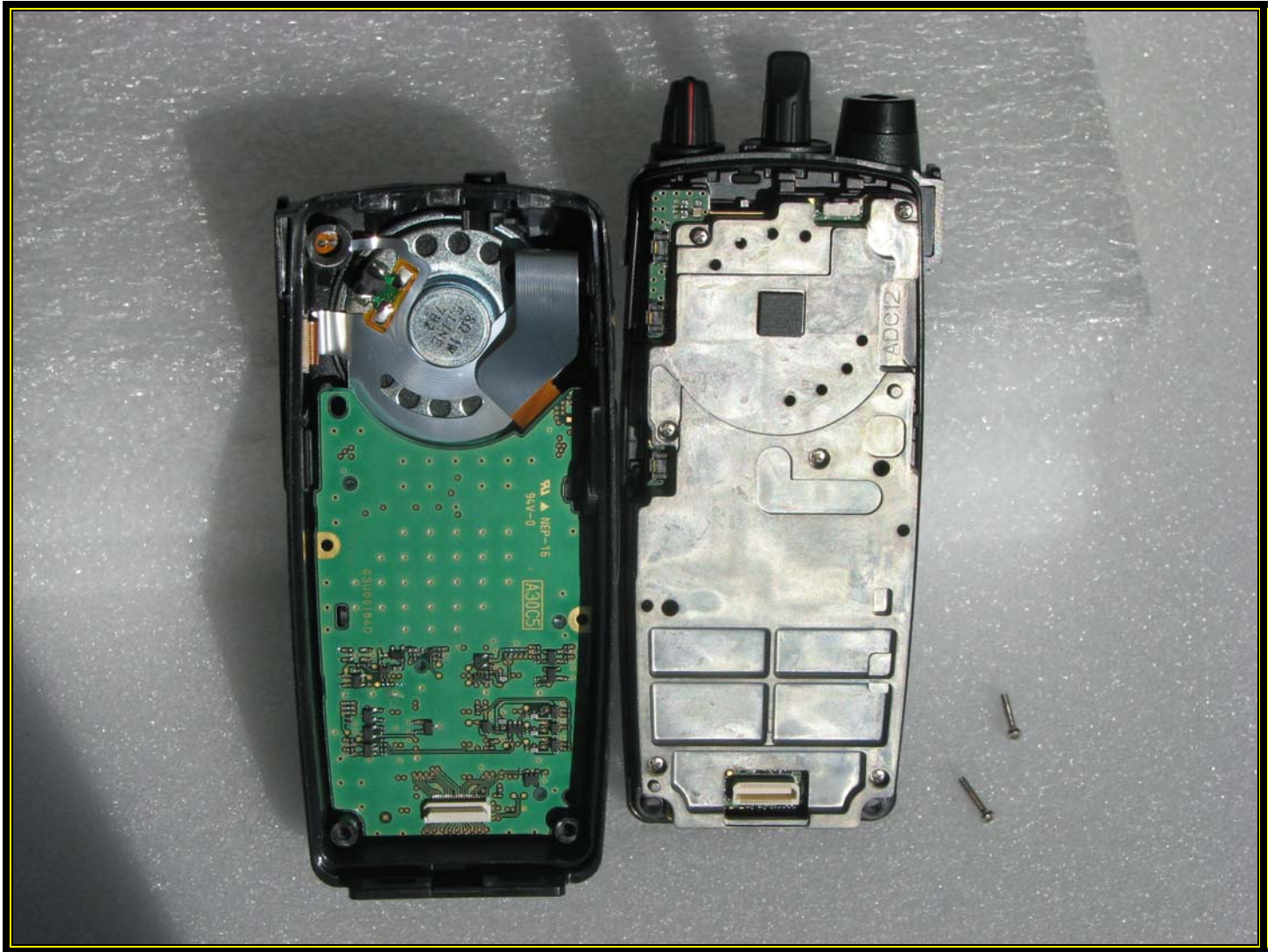
Photograph 11: Board Placement Layer 2
