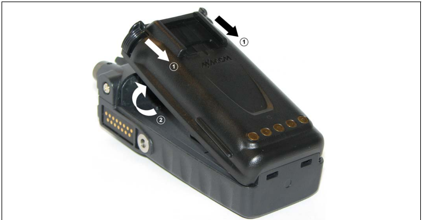
Figure 4-1: Removing the Battery Pack
