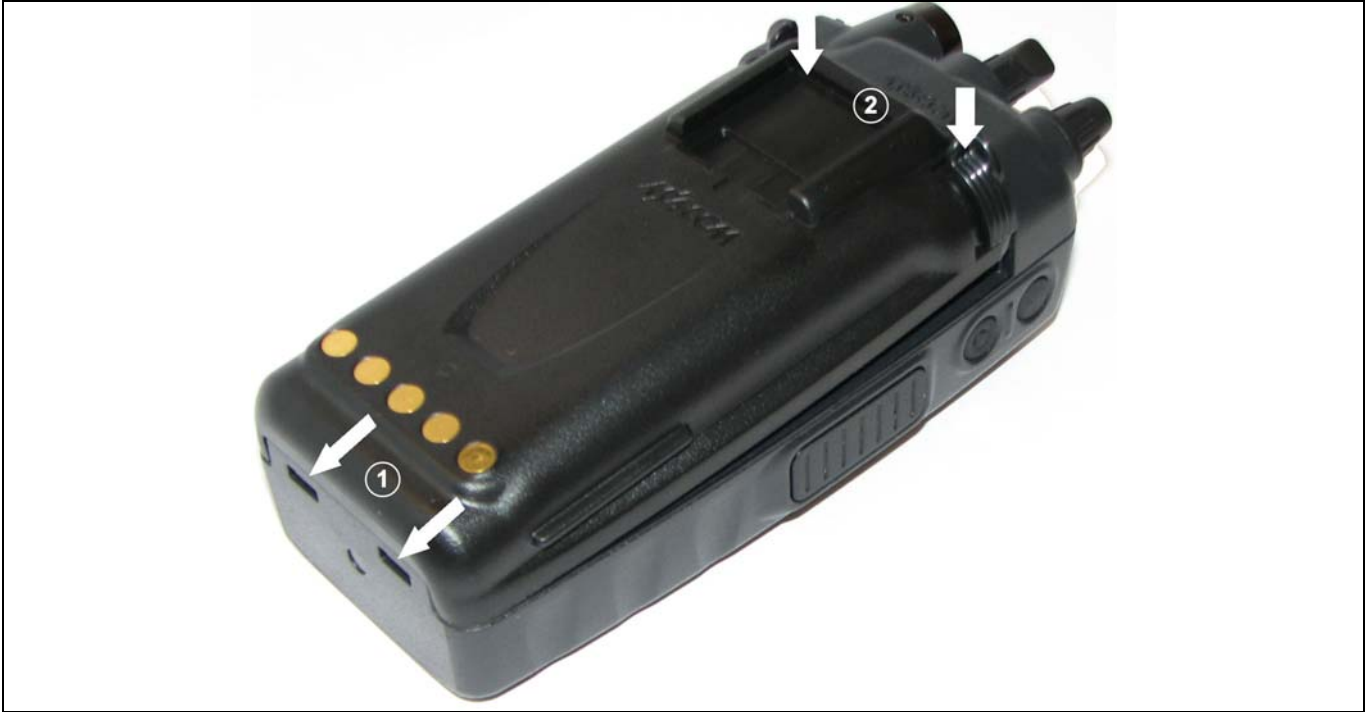
Figure 4-2: Attaching the Battery Pack
