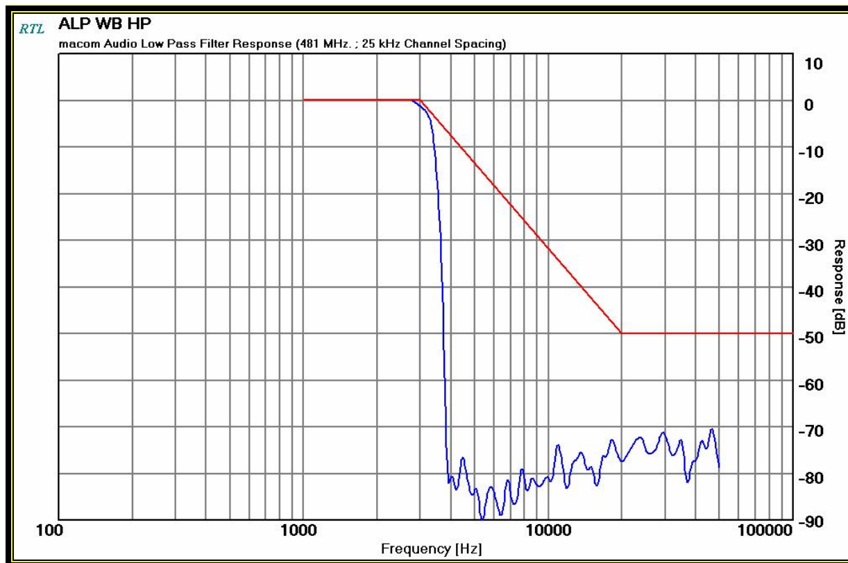
Plot 10-1: Modulation Characteristics – Audio Low Pass Filter; 815.5 MHz; Wide Band
