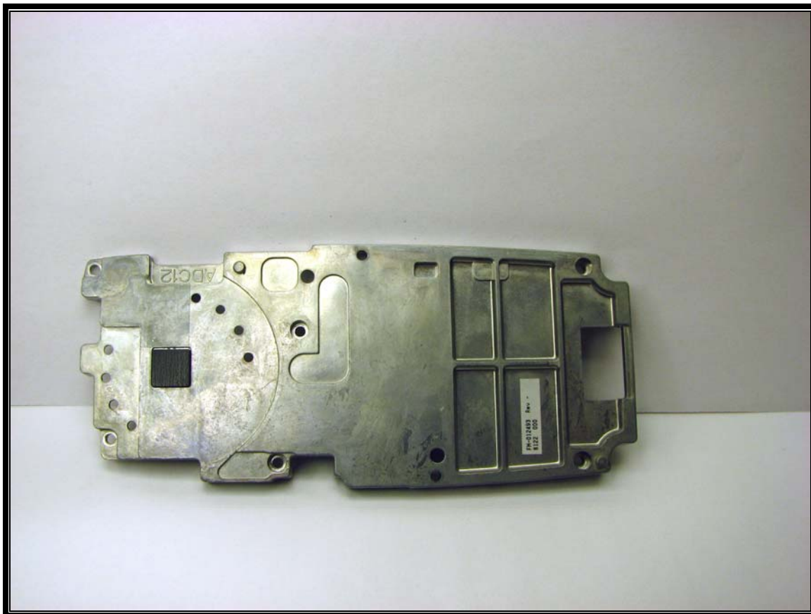
Photograph 13: RF Shield Top View
