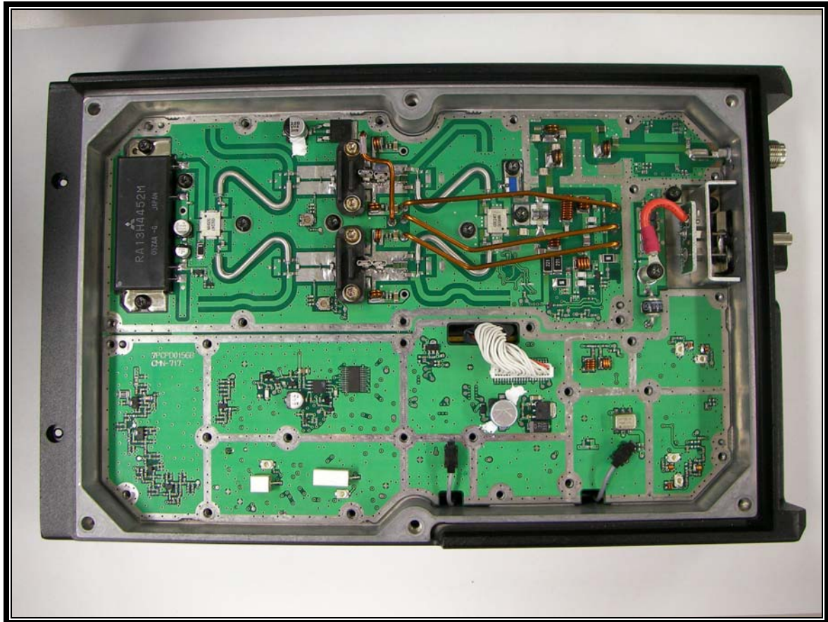
Photograph 16: Bottom Cover and Shield Removed2
