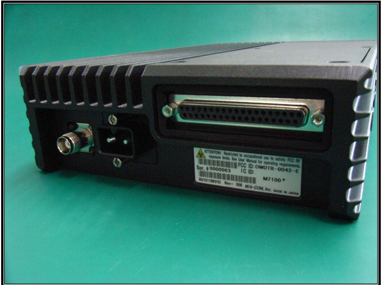
Photograph 2: Label Location on Rear of M7100
