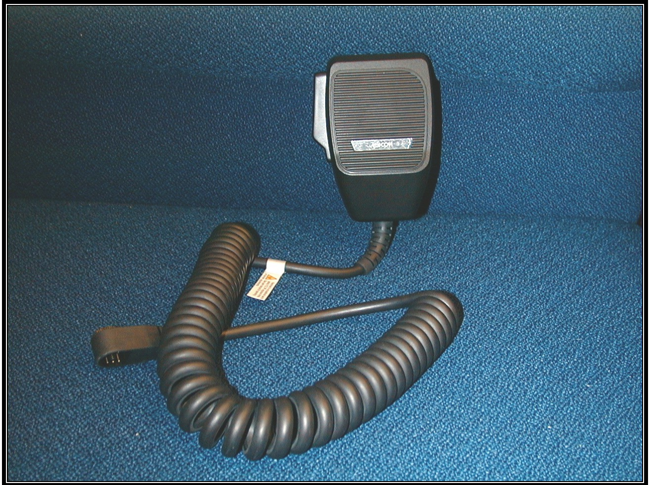
Photograph 4: RF Warning Label Location on Microphone
