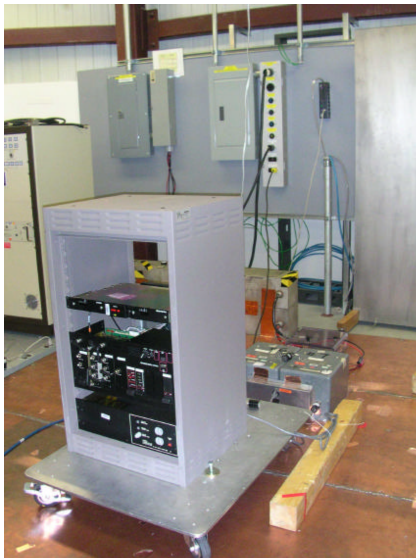
Figure 8-2: Conducted Emissions Test Set-Up
