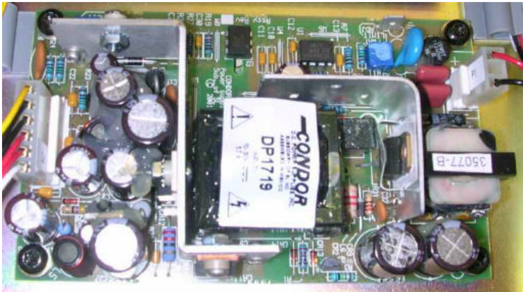
Figure 20: SitePro Power Supply Back
