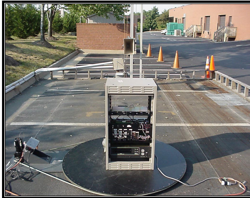
PHOTOGRAPH 1: RADIATED EMISSIONS FRONT VIEW
