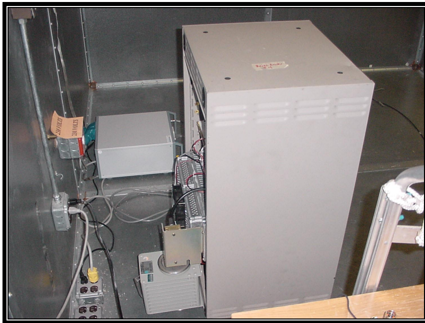
PHOTOGRAPH 4: Conducted Emissions Front View
