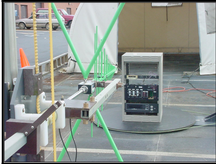
PHOTOGRAPH 1: Radiated Emissions Front View
