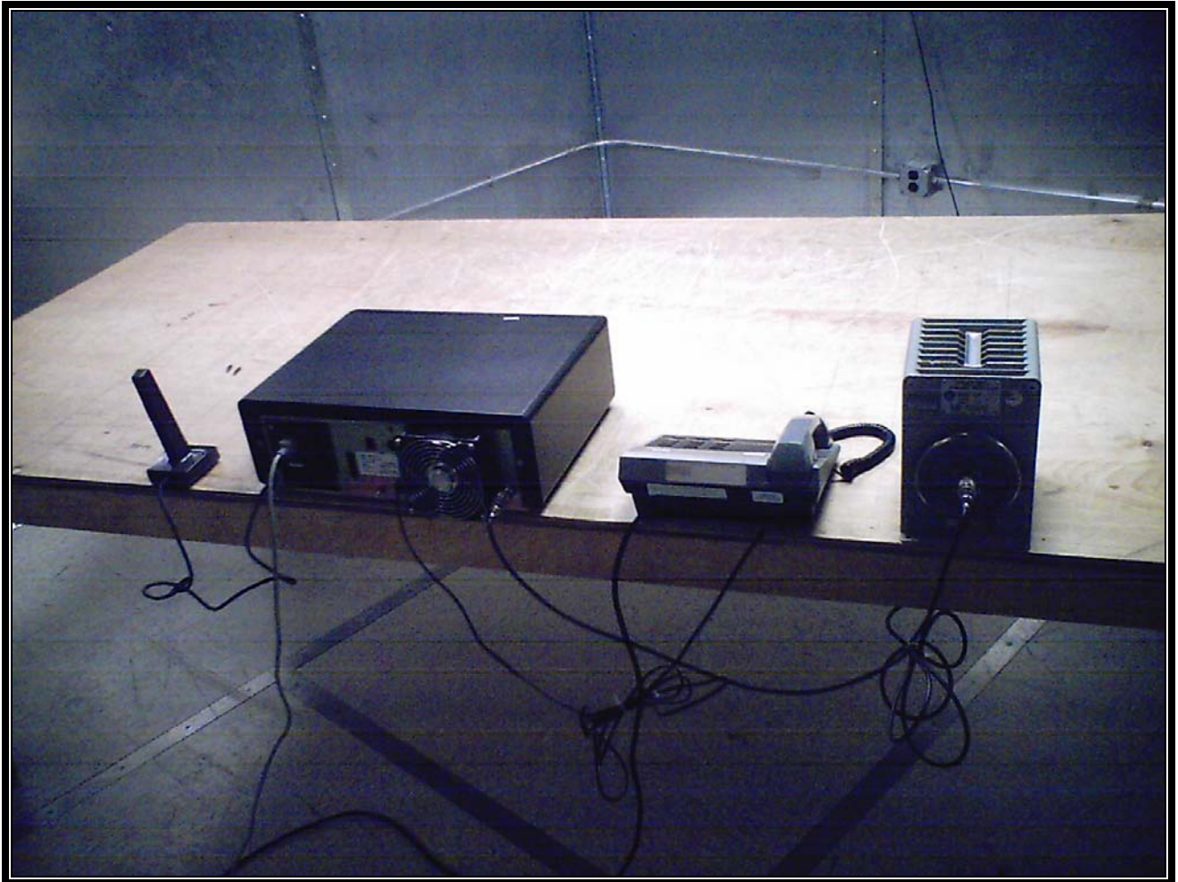
Photograph 8: Conducted Emissions (Rear View) Desktop Configuration
