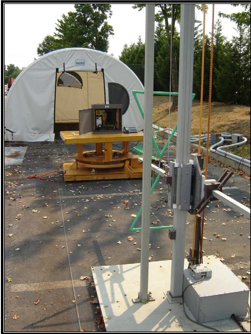
Photograph 1: Radiated Emissions (Front View) Wall Mount Configuration
