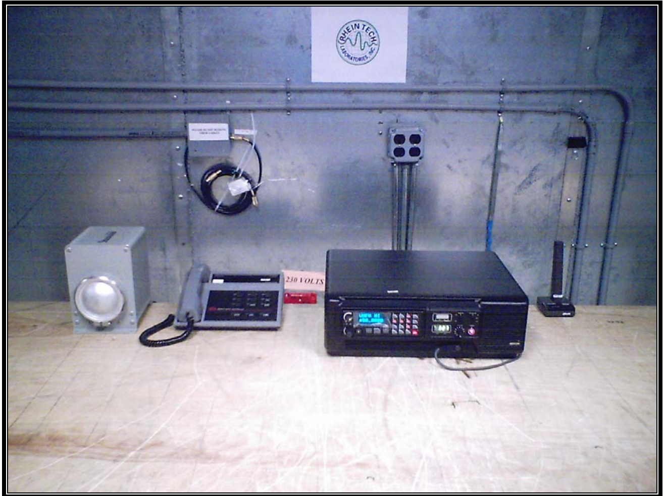
Photograph 7: Conducted Emissions (Front View) Desktop Configuration
