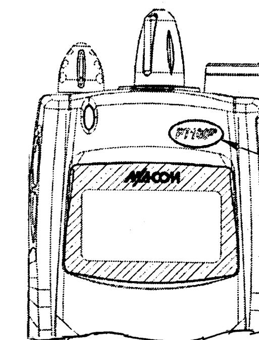
SVA23009/5 or equivalent P7100<sup>IP</sup> oval label on radio face installed by KDE
