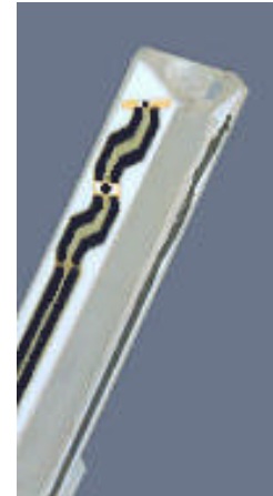
ET3DV6 E-Field Probe
