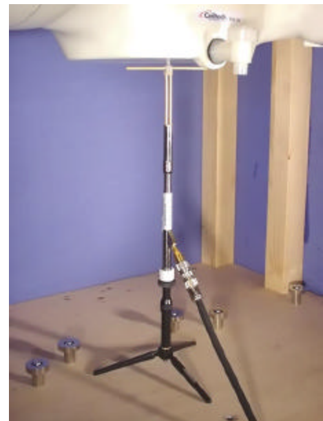
900MHz Dipole Validation Setup
