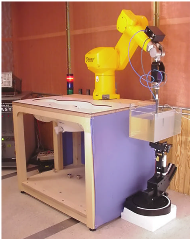
DASY3 SAR Measurement System with Planar Phantom
