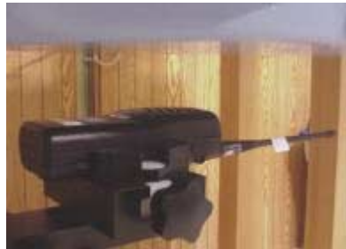
Face-held SAR Test Setup Antenna G Face-held SAR Test Setup Antenna I
