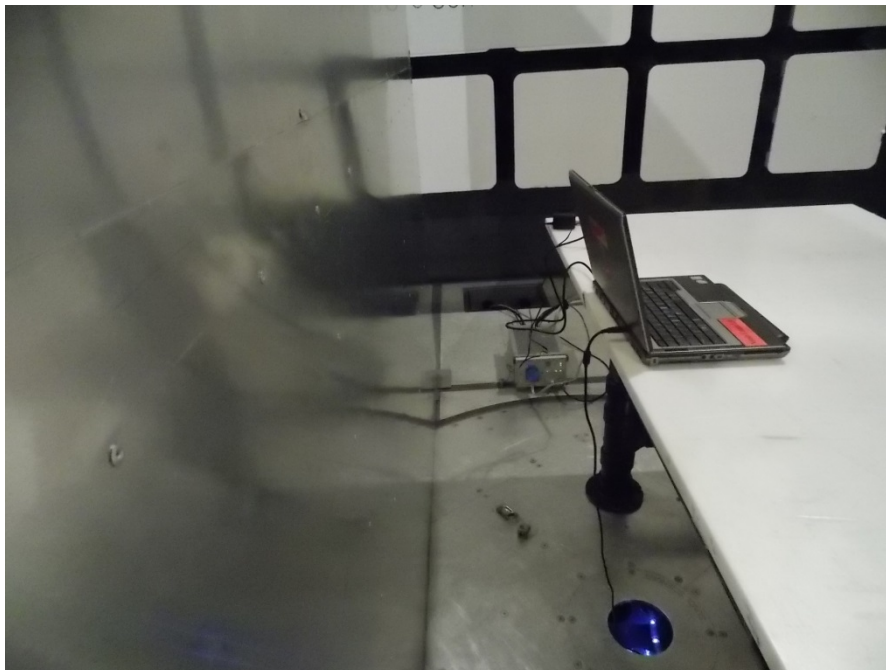
Figure 8.1-4: AC power line conducted emissions setup photo
