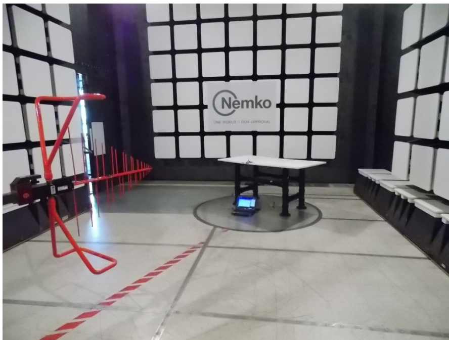
Figure 8.4-2: Spurious emissions (except for harmonics) setup photo
