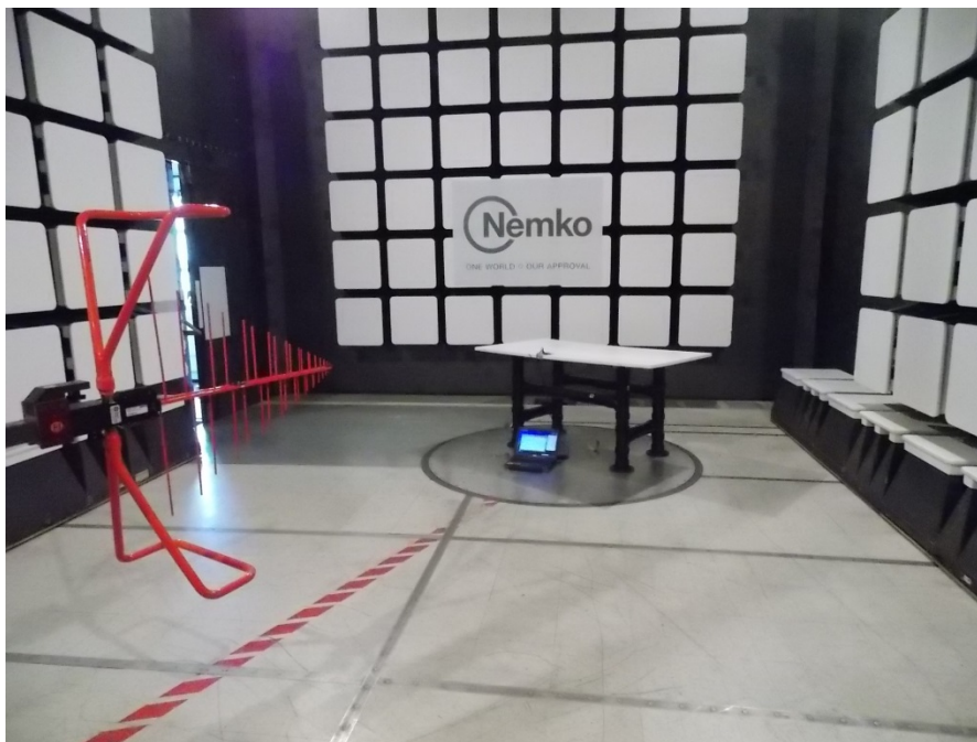
Figure 8.3-2: Field strength setup photo
