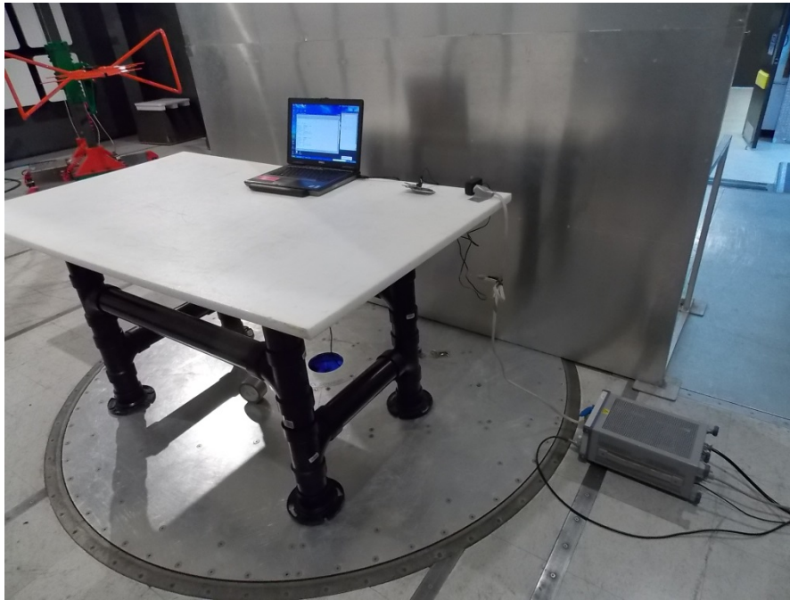
Figure 8.1-3: AC power line conducted emissions setup photo
