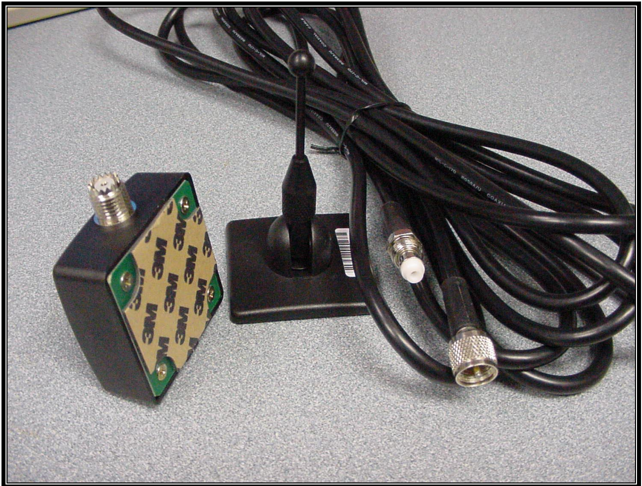
PHOTOGRAPH 11: 0DB GLASS MOUNT ANTENNA WITH CABLES AND CONNECTORS
