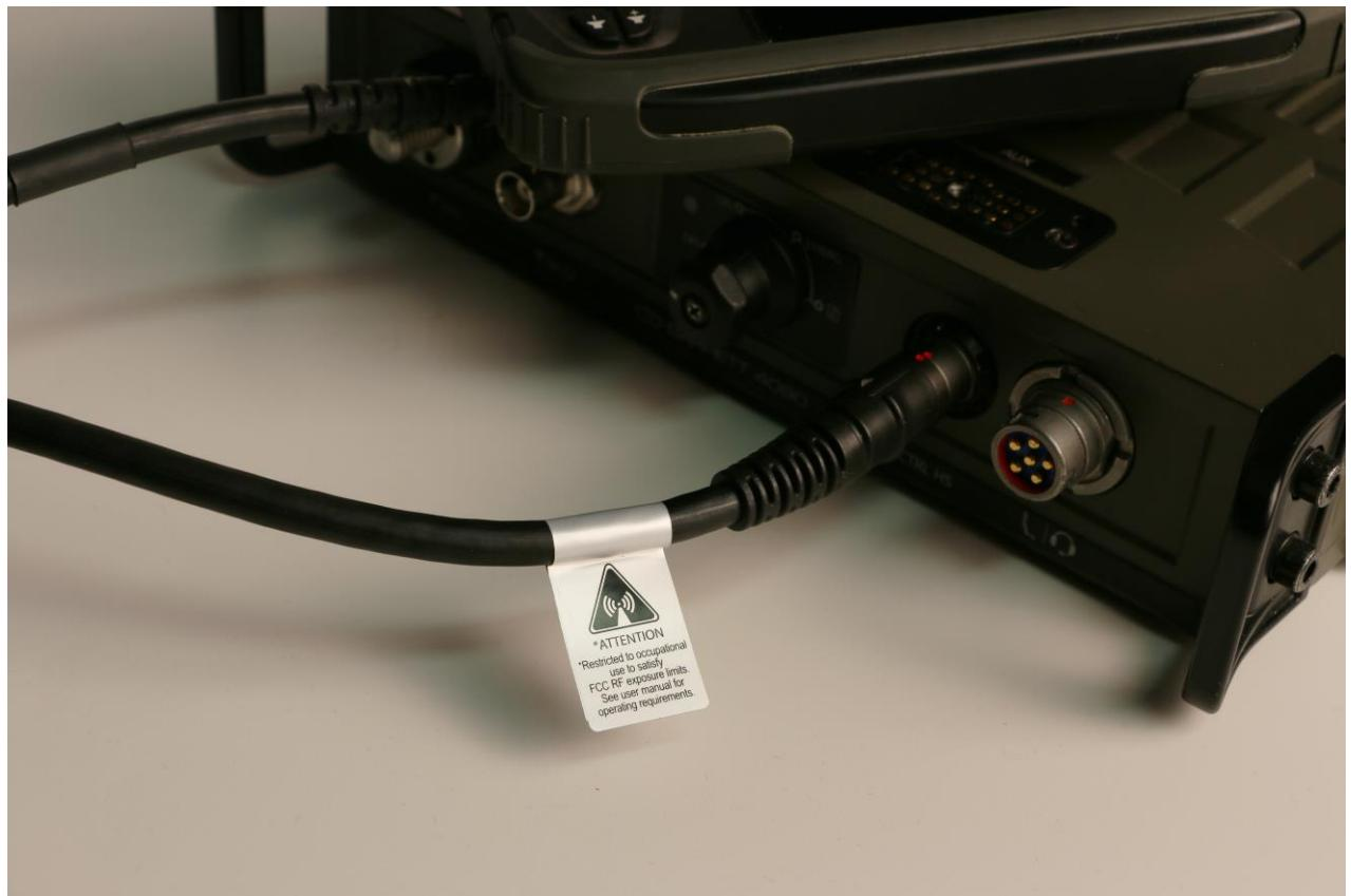
**Figure 4 – RF Exposure Warning Label Position**
