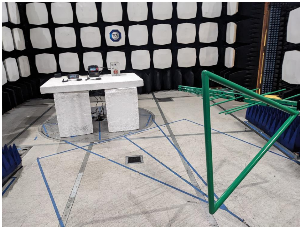
Figure A-3: Test Setup – Front View of the Radiated Emissions 30 – 500 MHz
