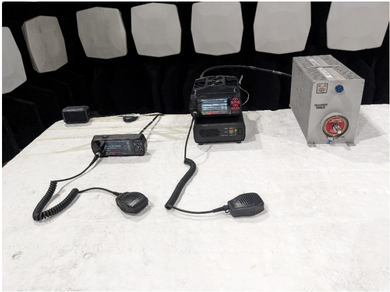
Figure 1.4.1-2 – Test setup of EUT with ancillaries
