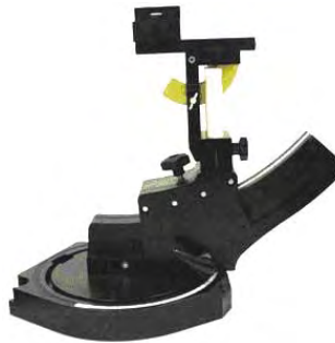
Device holder supplied by SPEAG
