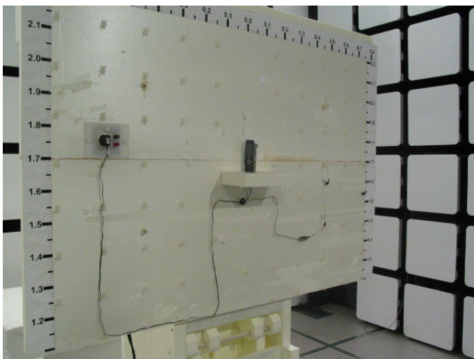
Picture 1 Spurious radiated emission measurement
