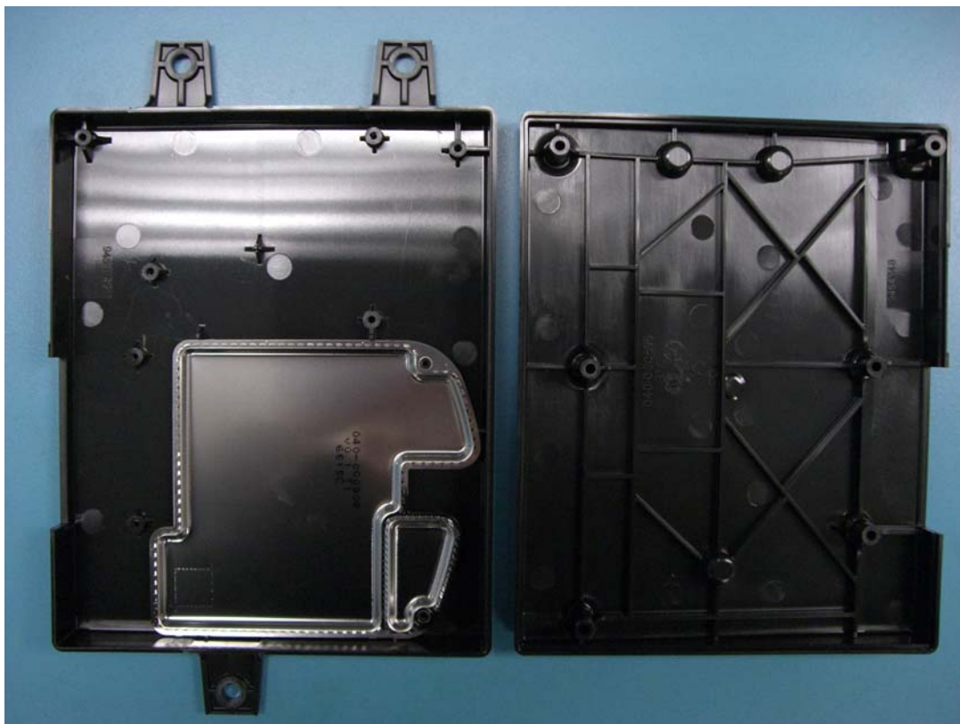
Mechanic with shielding only, without PWB
