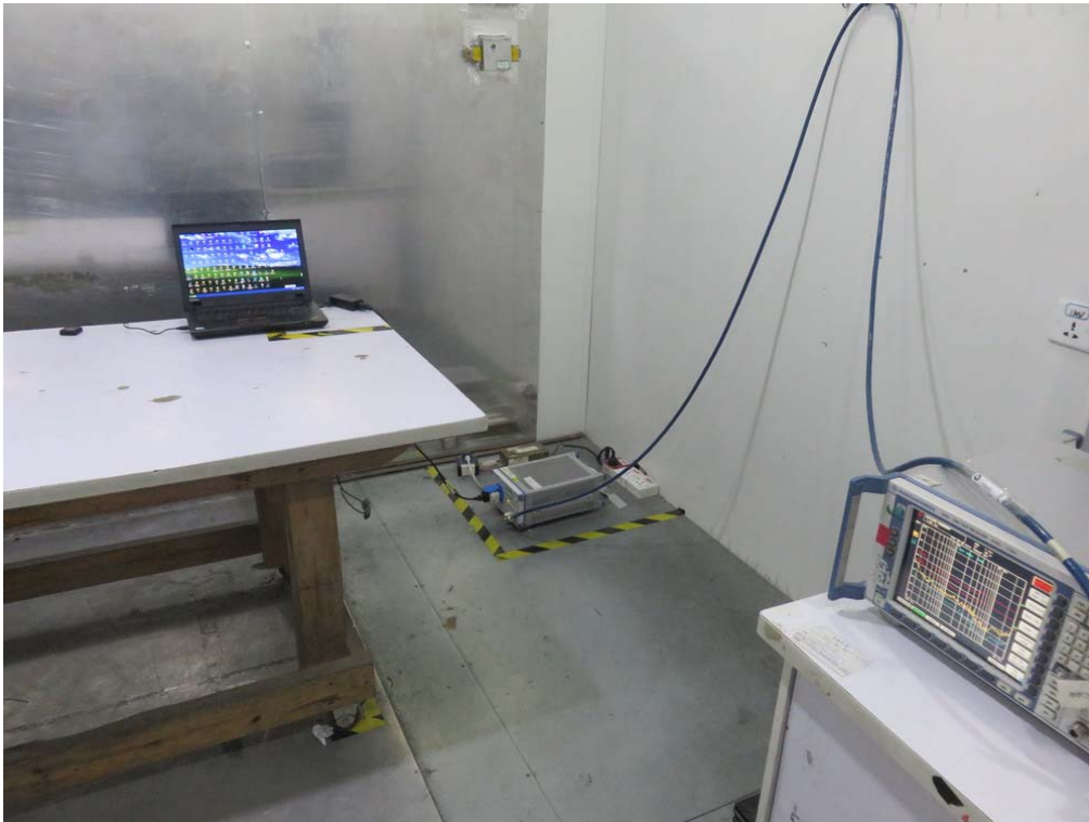
FCC RADIATED EMISSION TEST SETUP
