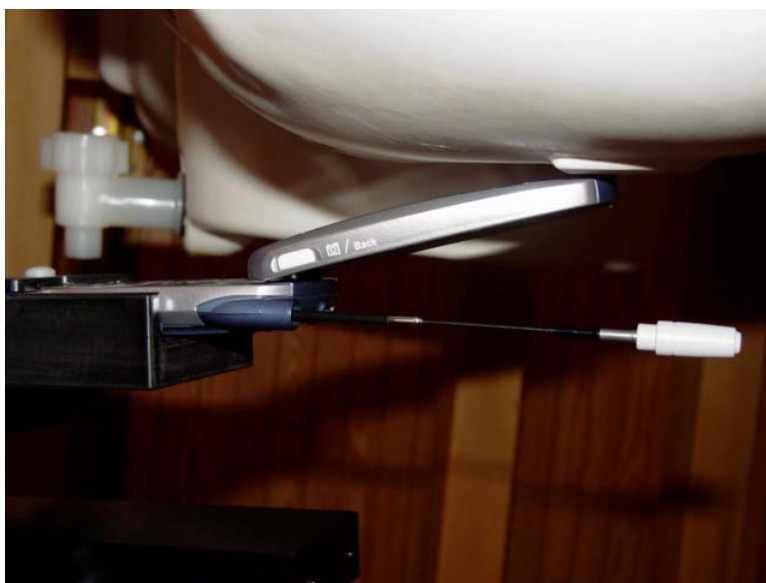
Figure 10.9 phone against the head (right tilt position, swivel open, antenna extended)
