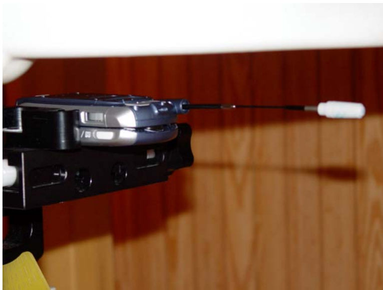
Figure 10.15 body SAR setup (with 25mm air separation, swivel closed, antenna extended)
