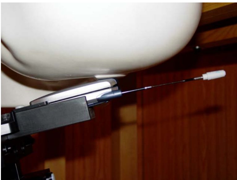
Figure 10.5 phone against the head (right tilt position, swivel closed, antenna extended)
