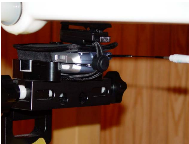
Figure 10.13 body SAR setup (with leather case, swivel closed, antenna extended)
