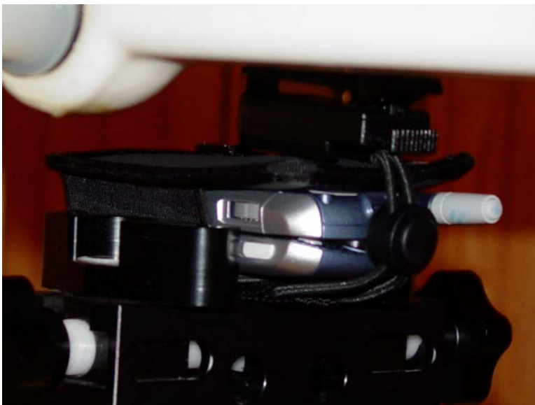
Figure 10.12 body SAR setup (with leather case, swivel closed, antenna retracted)
