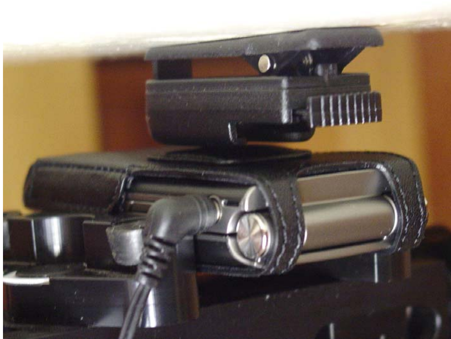
Figure 9E.5 Body SAR Phone setup Flip Closed with Leather Case (CV90-P0323-01)
