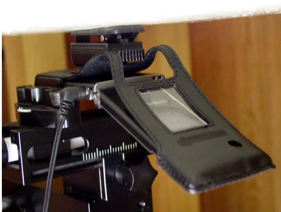
Figure 9E.6 Body SAR Phone setup Flip Open with Leather Case (CV90-P0323-01)
