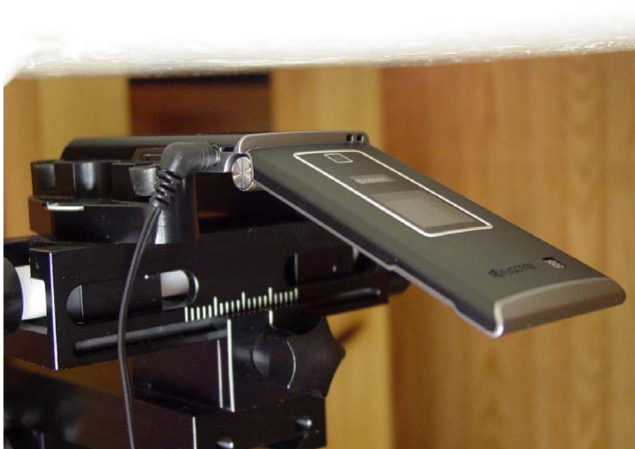
Figure 9E.4 Body SAR Phone setup Flip Opened (15 mm Air Separation)
