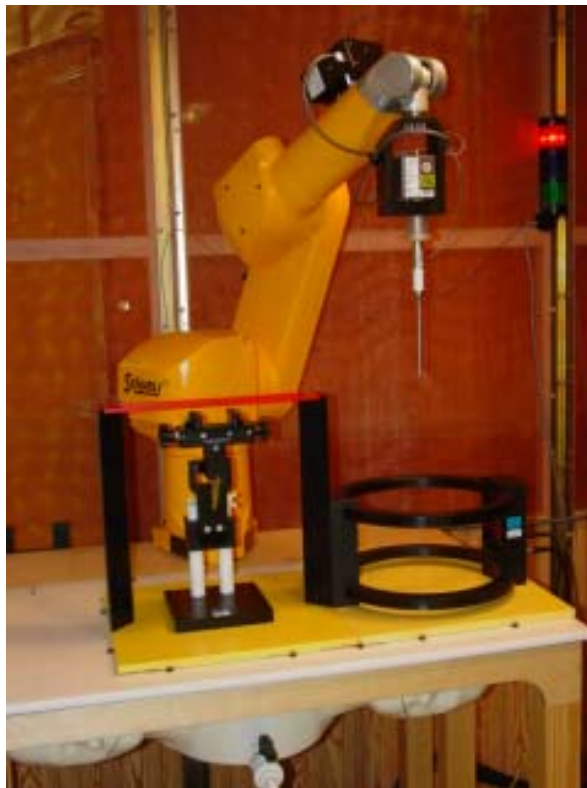
Figure 5.2a T-Coil setup with Helmholtz Coil
