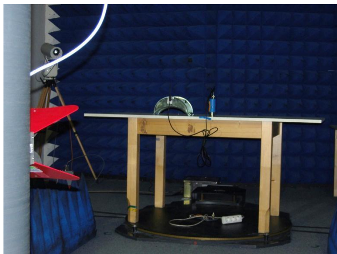
Dipole antenna with cable extension
