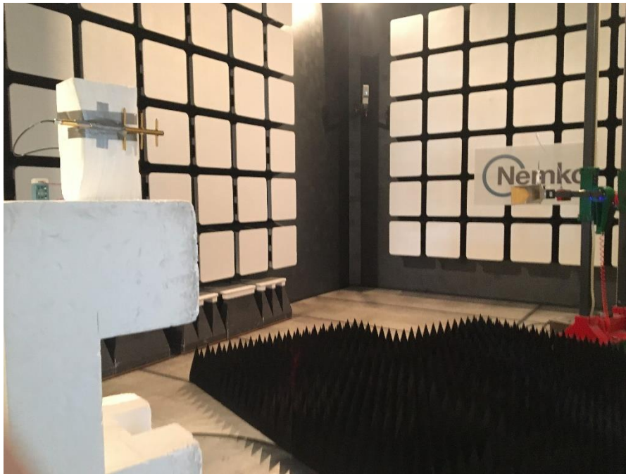
Figure 1.1-8: Radiated emissions setup photo – above 1 GHz (Yagi antenna, MN: Y8963)
