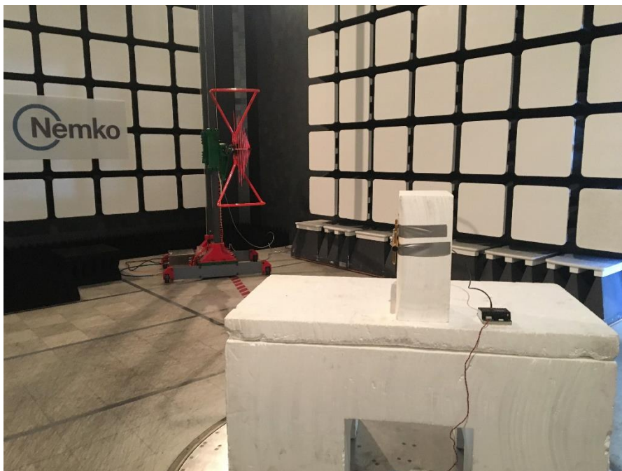
Figure 1.1-4: Radiated emissions setup photo – below 1 GHz (Yagi antenna, MN: Y8963)
