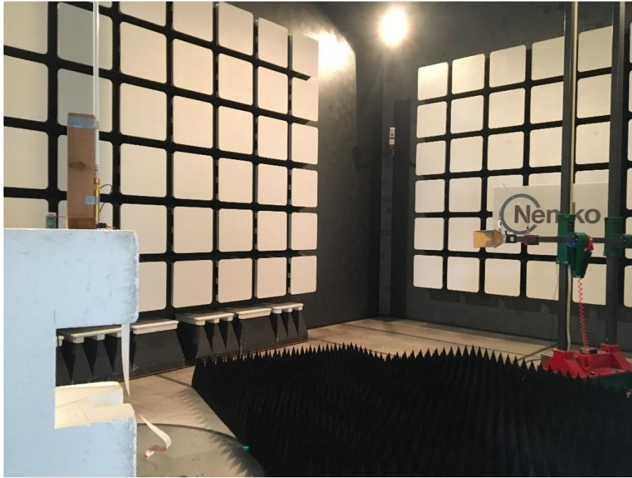
Figure 1.1-5: Radiated emissions setup photo – above 1 GHz (Rod Antenna, MN: FG9026)
