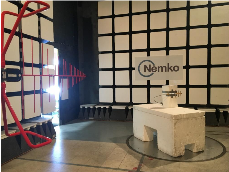
Figure 1.1-3: Radiated emissions setup photo – below 1 GHz (Yagi antenna, MN: Y8963)
