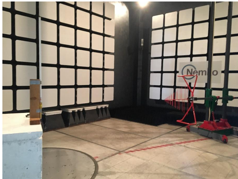
Figure 1.1-2: Radiated emissions setup photo – below 1 GHz (Rod Antenna, MN: FG9026)
