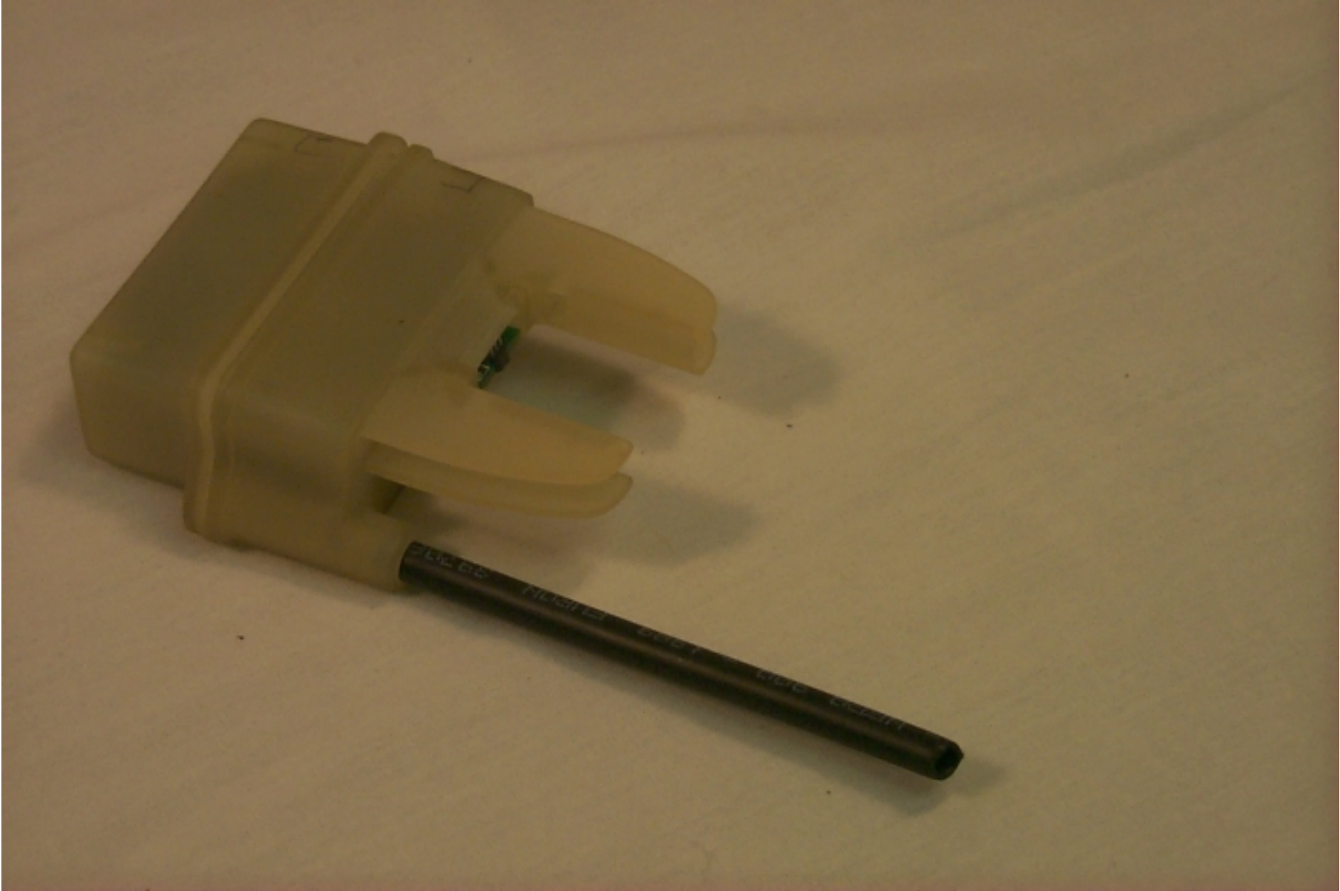
Saar Associates Model: WMS (Water temperature and flow meter transmitter)
