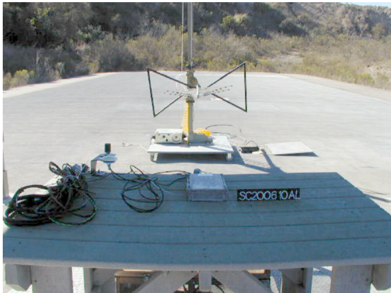
Photograph of Test Setup: Radiated Emissions
