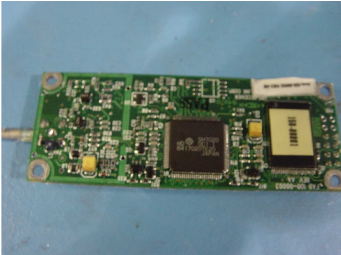
GPS module with RF shield removed (top)
