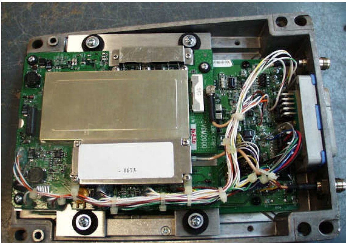
Deere ra with top half of enclosure removed showing Communications Interface PCB – view
