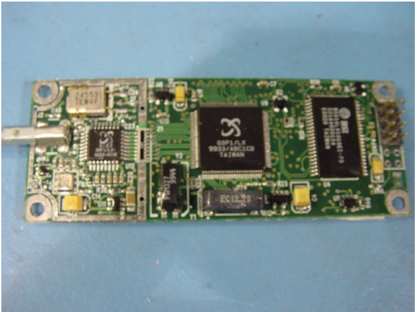
GPS module with RF shield removed (bottom)
