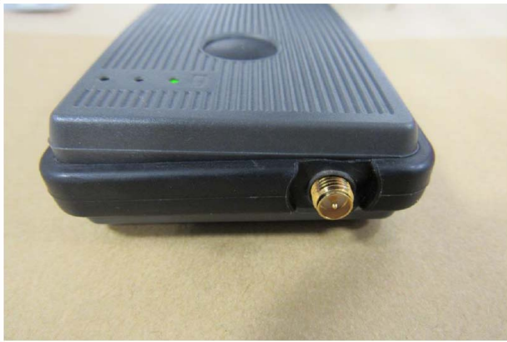
EUT ANTENNA CONNECTOR
