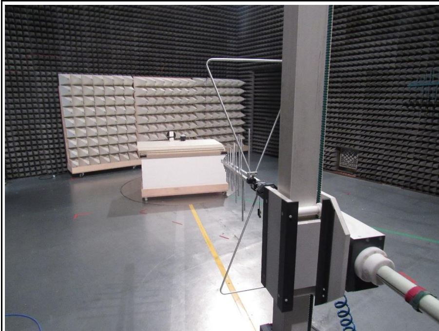
Setup for measurements below 1 GHz (Pit Antenna)
