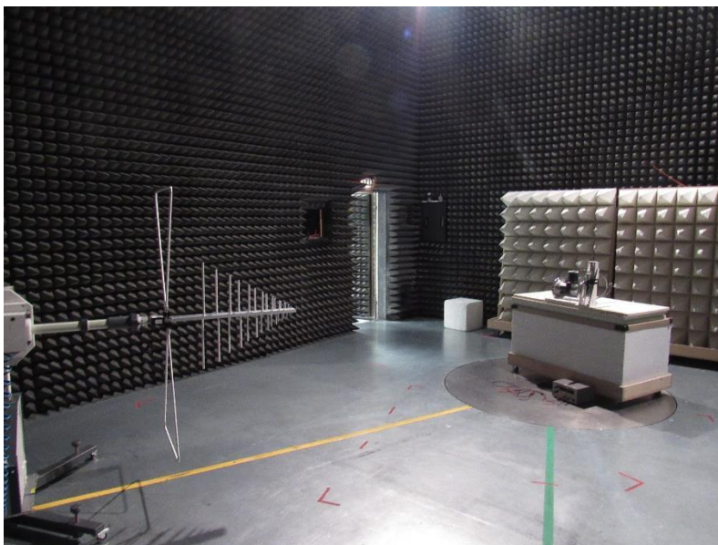
Wall antenna - < 1 GHz
