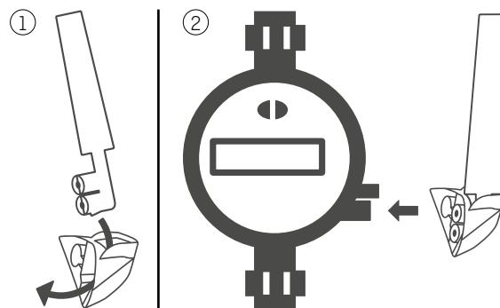
Step 1: Push the base of the helix antenna through the seal housing.
