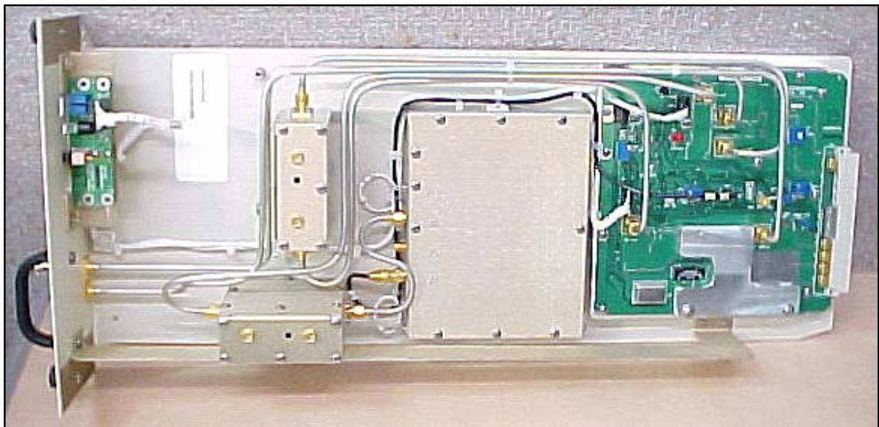
**6.5 Side view - Control / Power Supply Assembly (Exciter)**
