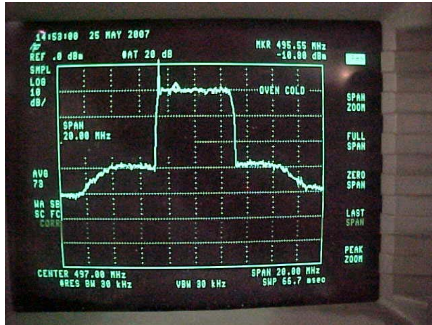
Figure 4B-8A. Reference (497 MHz) = -1 dBm (Pre-Filter)
