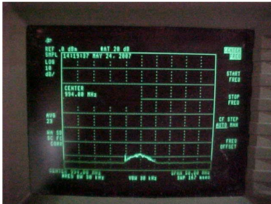
Figure 4B-8B. Second Harmonic (994 MHz) = -70 dBm (Pre-Filter)
