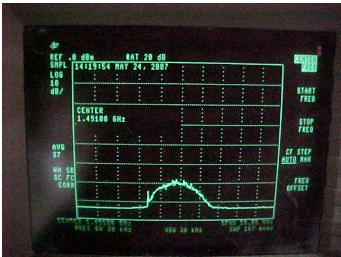
Figure 4B-8C. Third Harmonic (1491 MHz) = -61 dBm (Pre-Filter)
