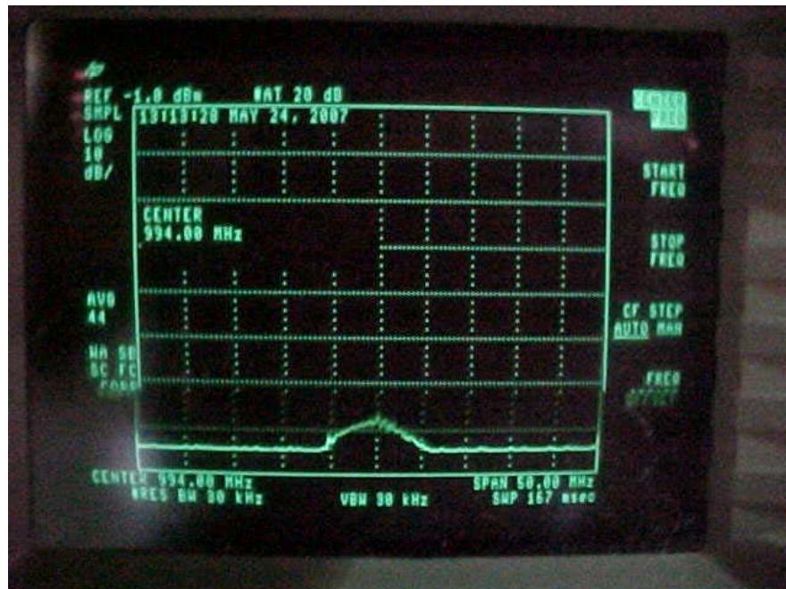
Figure 4A-8B. Second Harmonic (994 MHz) = -70 dBm (Pre-Filter)
