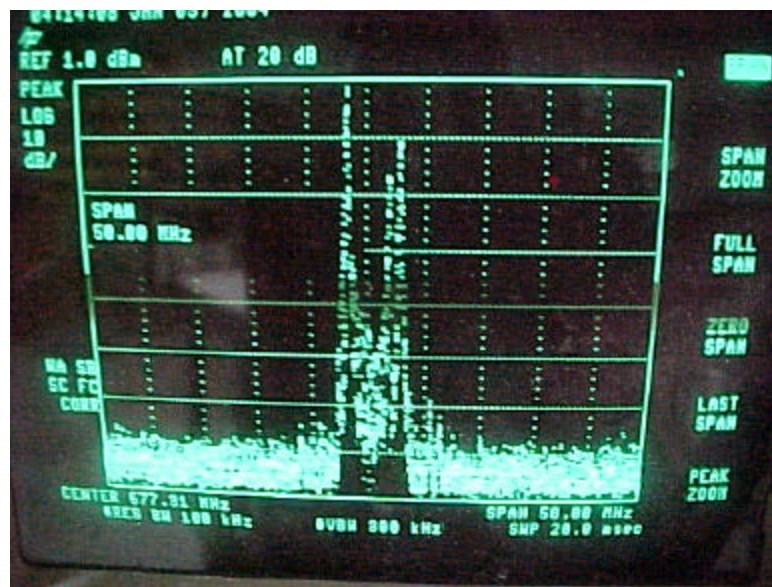
Figure 4-9. Products Above the 70 dB Noise Floor of the Spectrum Analyzer (1 of 2)
