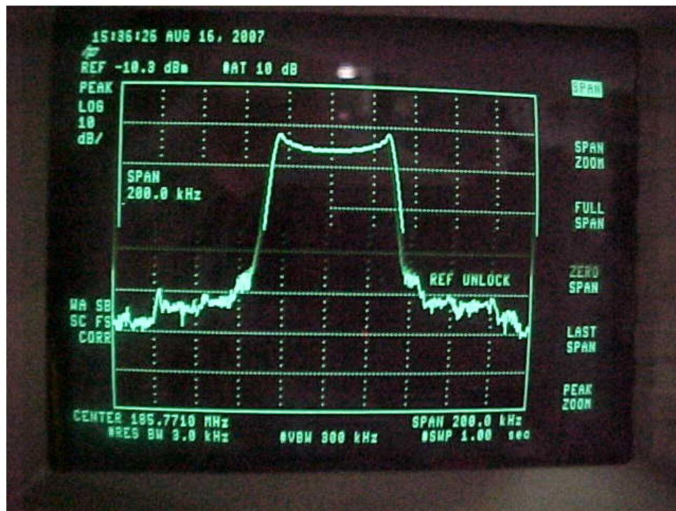
Figure 4-8. Aural Carrier-Occupied Bandwidth
