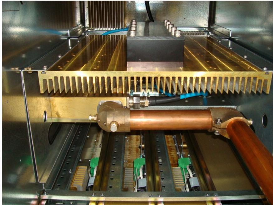
**6.11 Side view – PA Power Supply Assembly x2 (RF Amplifier Cabinet)**
