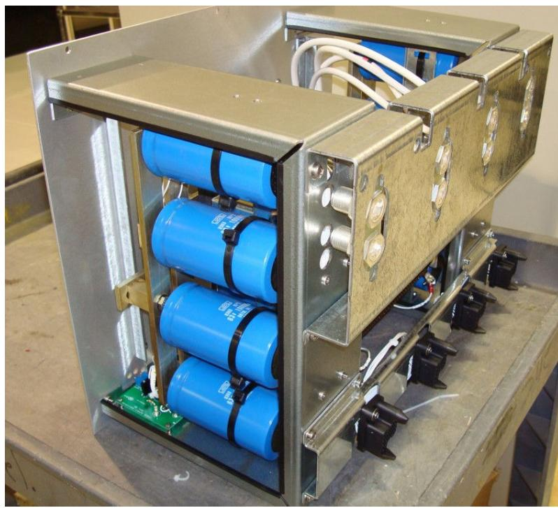
**6.12 Front view – AC Power Supply Assembly x2 (RF Amplifier Cabinet)**
