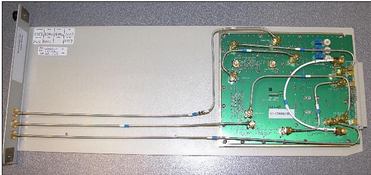
**6.4 Side view - Control / Power Supply Assembly (Exciter)**
