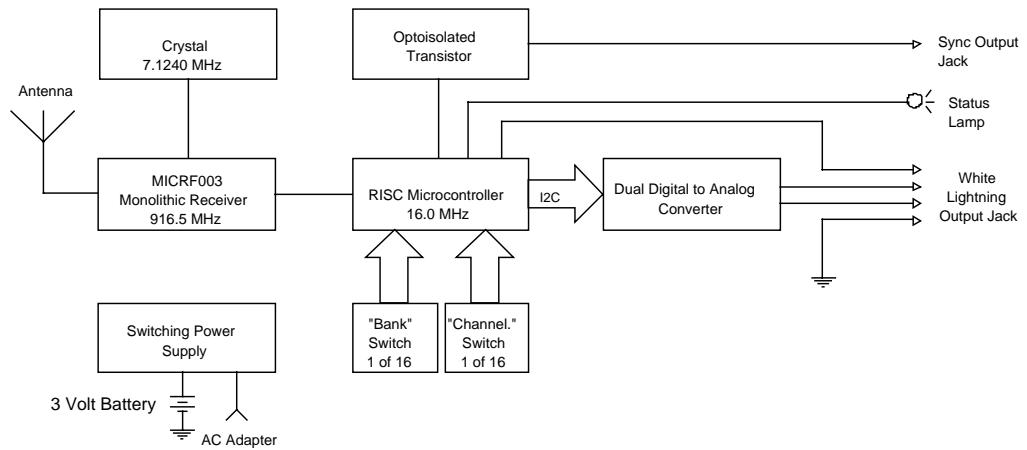
**Figure 1 RR1RX Block Diagram**
