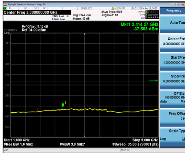
Band13-5MHz-QPSK-23255-1-0-High-1000-5000--37.58-PASS
