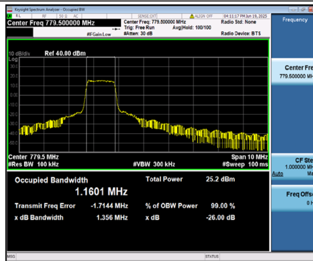
Band13-5MHz-QPSK-23205-6-0-Low-1.1601-1.160-PASS
