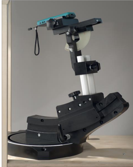
F-2. Device Holder for Transmitters
