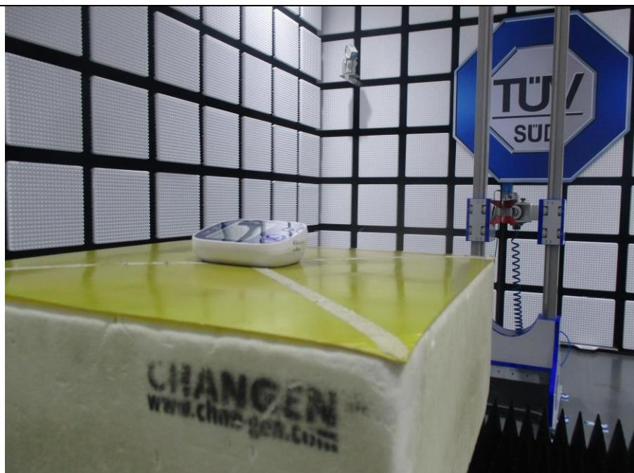
Details of: Radiated Emission test (above 18GHz)
