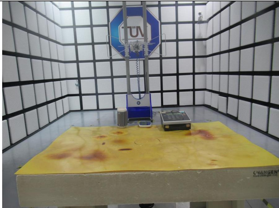
Details of: Radiated Emission test (1-18GHz)
