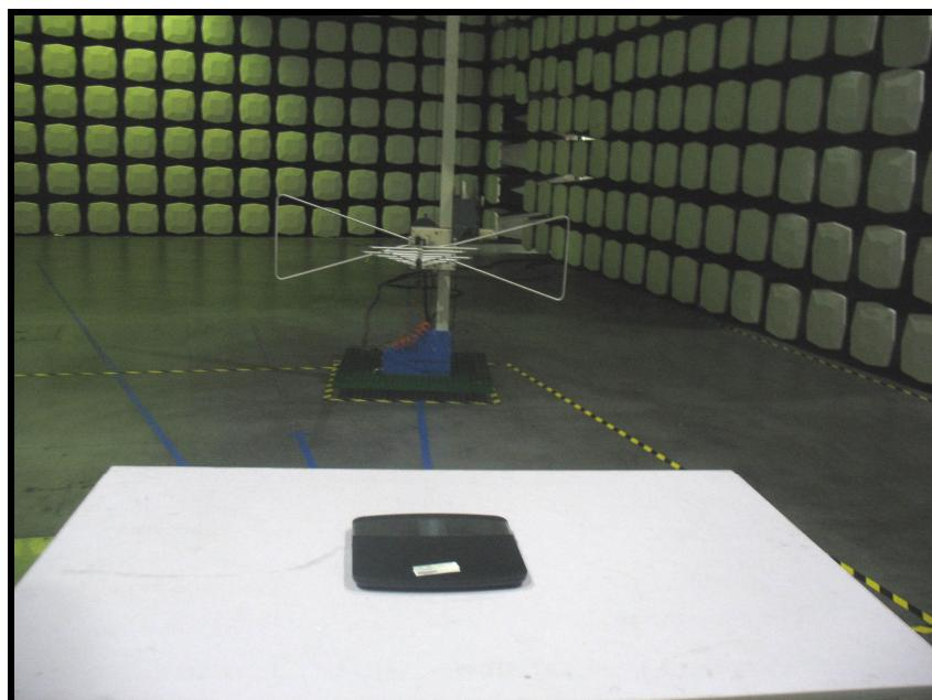
Above 1GHz: (full anechoic chamber)
