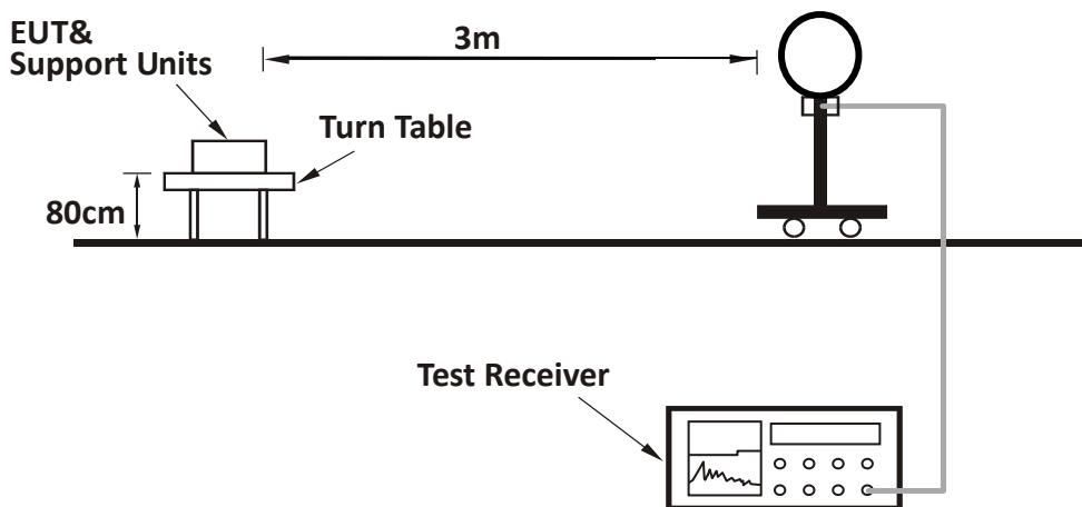
For Radiated emission 30MHz to 1GHz:
