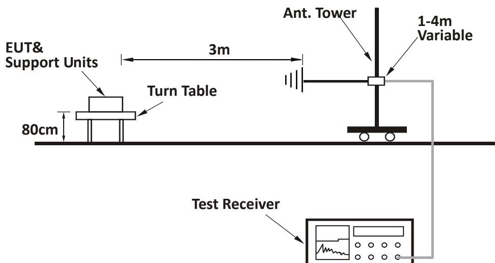
**TEST REPORT****For Radiated emission above 1GHz:**
