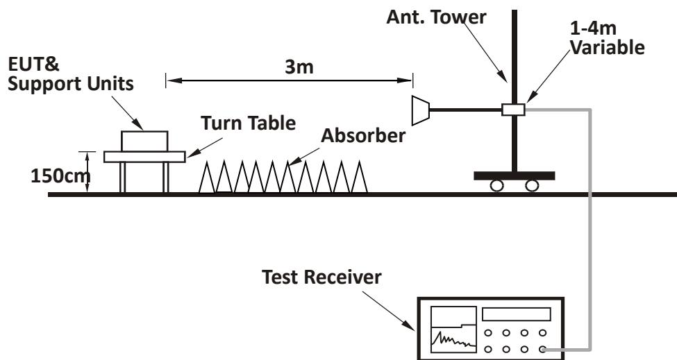
**TEST REPORT****7.4 Test Results of Radiated Emissions**
